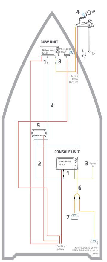
Minn Kota Trolling Motor with i-Pilot Link Built in MEGA Down Imaging and (1) bow-mounted Humminbird unit and (1) console-mounted Humminbird unit
